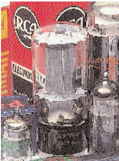
Valve heaven: an original RCA 'black plate' 6L6GC
